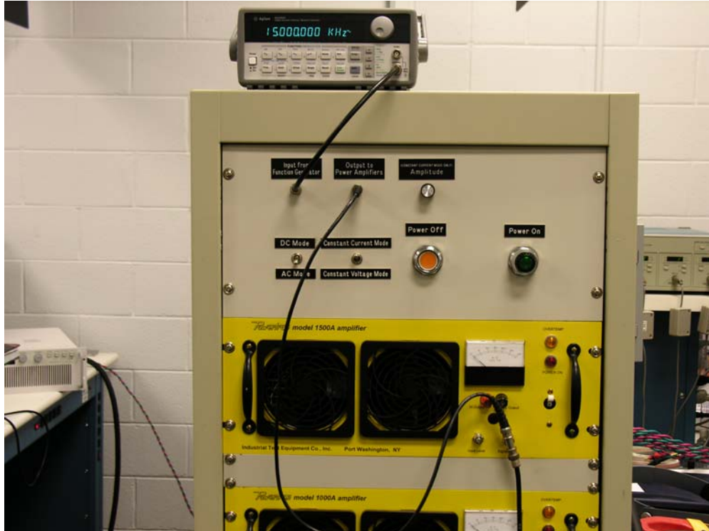
Fig. 2.1. An ac amplifier and signal generator used to produce ripple current.
