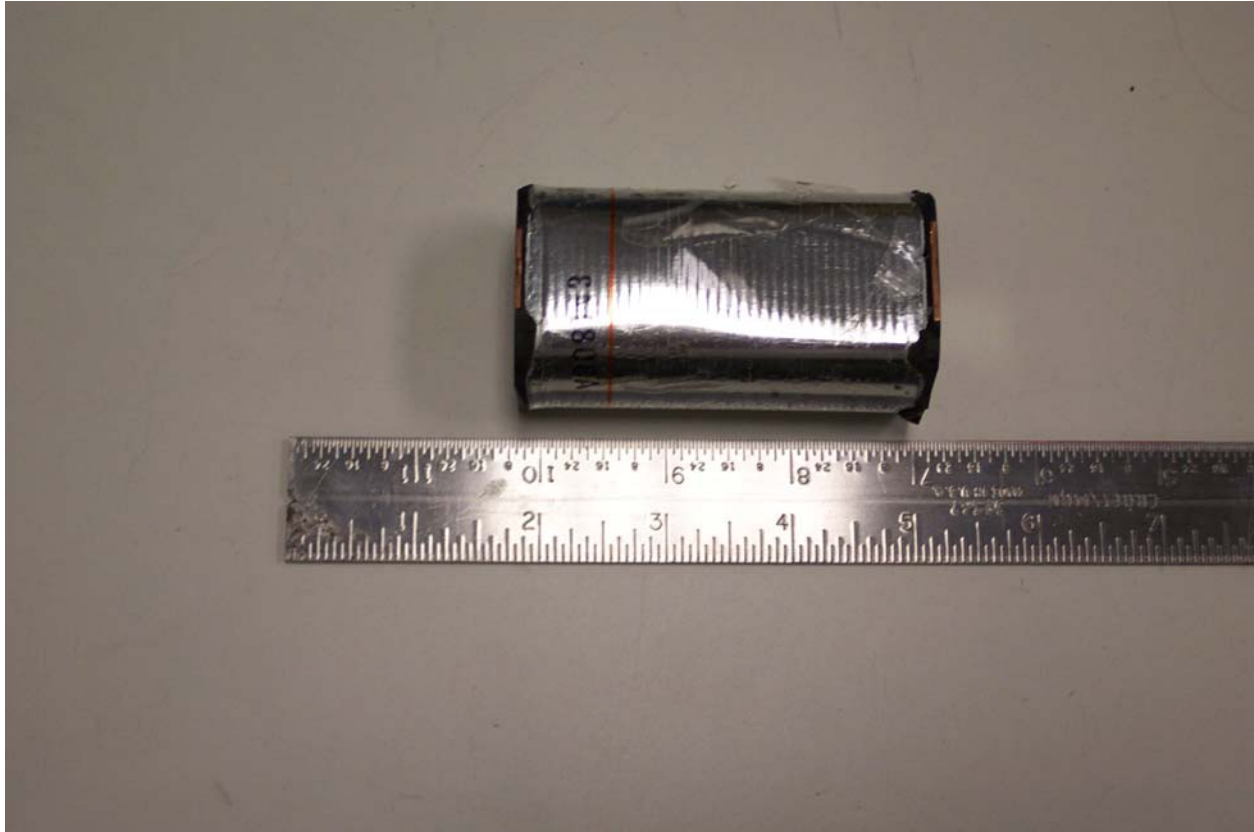
Fig. 3.2. A single Prius 140 uF 600 Vdc film capacitor.
