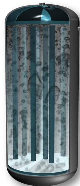
Figure 1. Churn-turbulent three-phase flow in a SBCR.
