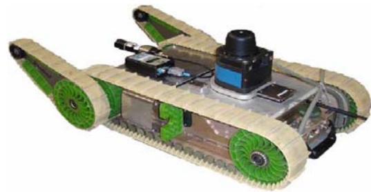
Fig. 7. The iRobot Packbot that was augmented with INL navigation payload and radiation sensor and used in Experiment 1.
