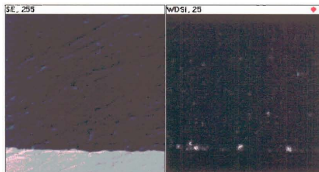
Figure 9. SEM photomicrograph (left) and EDX elemental mapping (right) of the monolithic fuel-clad interface of a 25.4 \mu\text{m} thick Al-2Si thermal spray coating after FB. The dark region is the Al cladding and the light region is the monolithic fuel.
