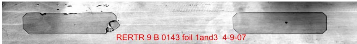
Figure 5. UT scans of an assembly fabricated employing a tool face from Alloy B for the RERTR-9B irradiation campaign.
