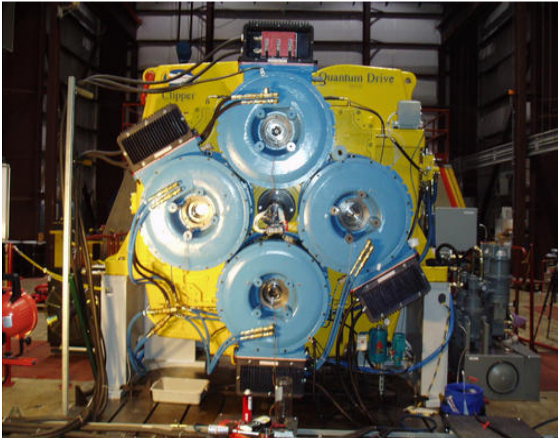
FIGURE 11. Clipper Windpower's distributed drive train.
