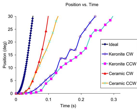
Figure 5: Typical time vs. position results for the tilt axis.
