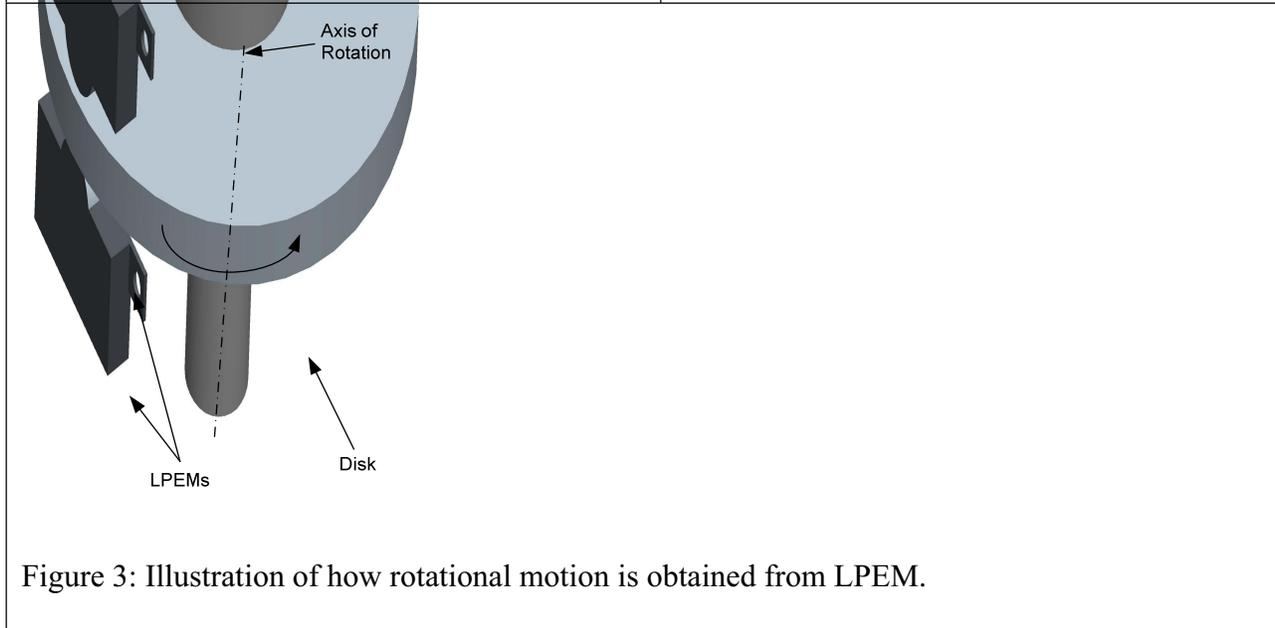
Figure 3: Illustration of how rotational motion is obtained from LPEM.
