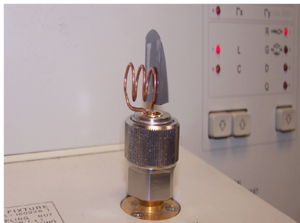
Figure 1. Photograph of sample (wafer piece) coupled to coil antenna and mounted on an impedance analyzer.
