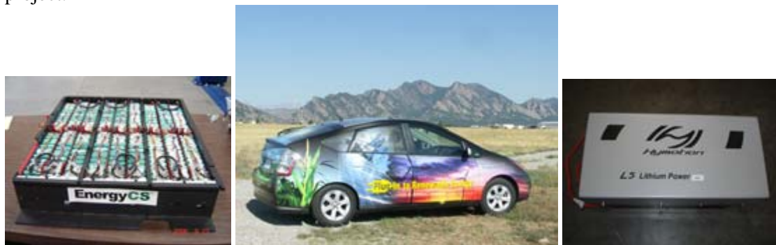
Figure 1: NREL PHEV Test Bed (2006 Toyota Prius, 9kWh and 5kWh PHEV Battery Packs)
