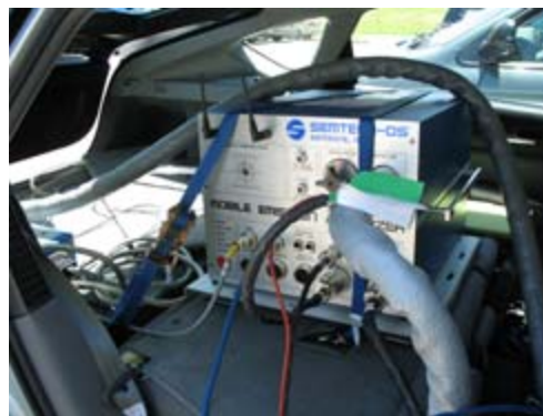
Figure 4: SEMTECH-DS installed in rear of NREL PHEV
