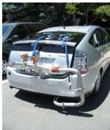
Figure 3: PEMs Exhaust Flow Meter (2" diameter) attached to NREL PHEV
