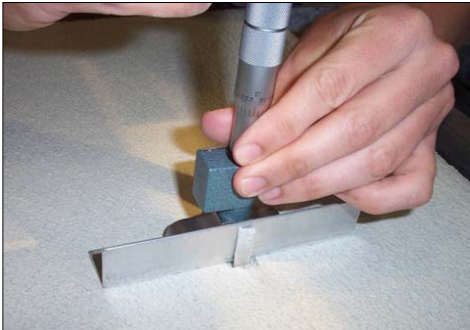
Figure 16: Measuring coating thickness during pilot production.
