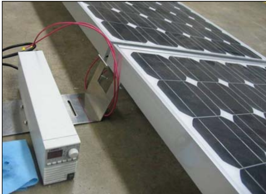
Figure 28: Grounding test on an RFT10 assembly.
