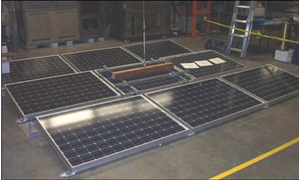
Figure 27: Uplift test on RFT10 tiles with vertical force is applied to the center tile.
