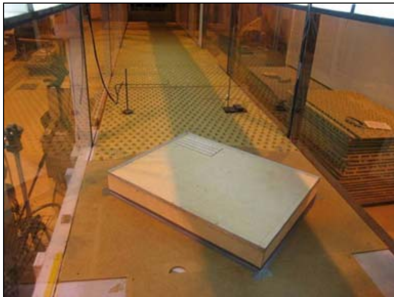
Figure 24: Wind tunnel model for an RFT10 array installed on the edge of a building.
