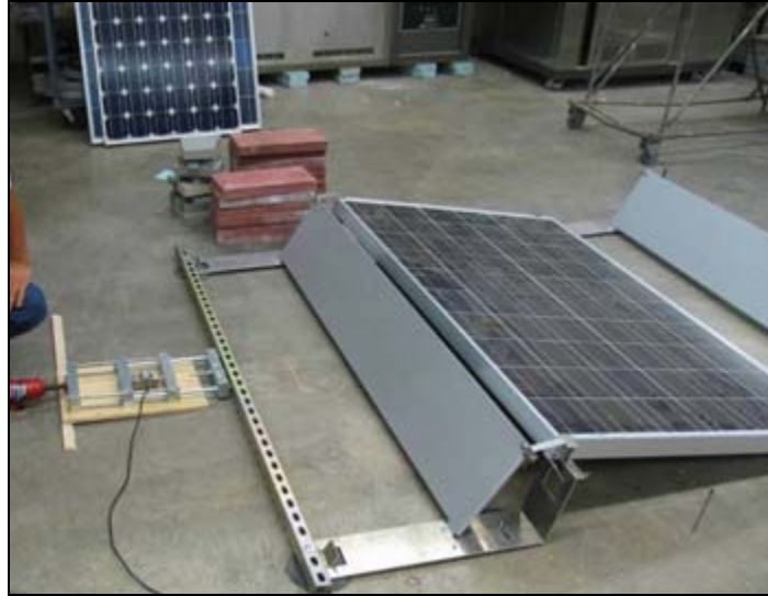
Figure 25: Lateral load test on RFT10 assembly. A compressive load is applied to the north side of the tile.
