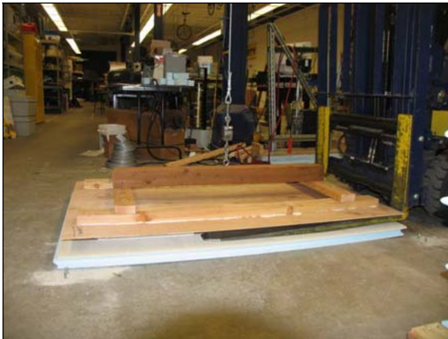
Figure 20: Tensile test of PowerGuard tile made with continuous process.
