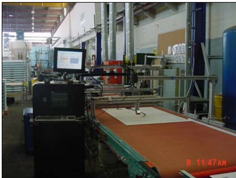
Figure 38: PV preparation line, showing operator station and bar-code scanner.
