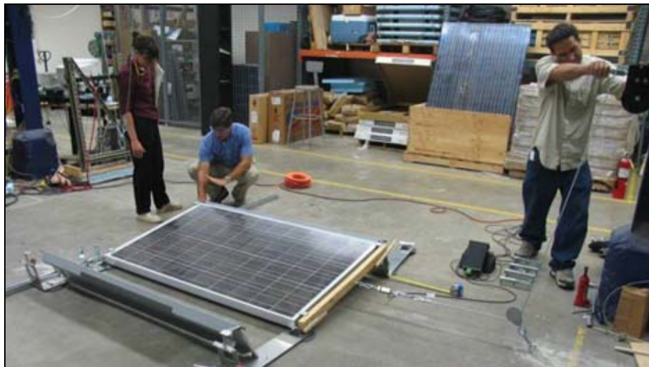
Figure 26: Lateral load test on an RFT10 assembly. A tensile load is applied to the east side of the assembly.
