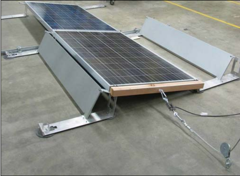
Figure 30: Lateral load test on RFT10 universal design.
