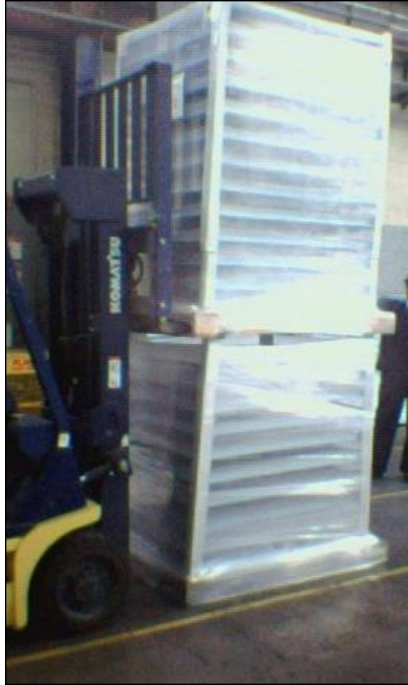
Figure 41: Test of corner supports in double stacked pallets.
