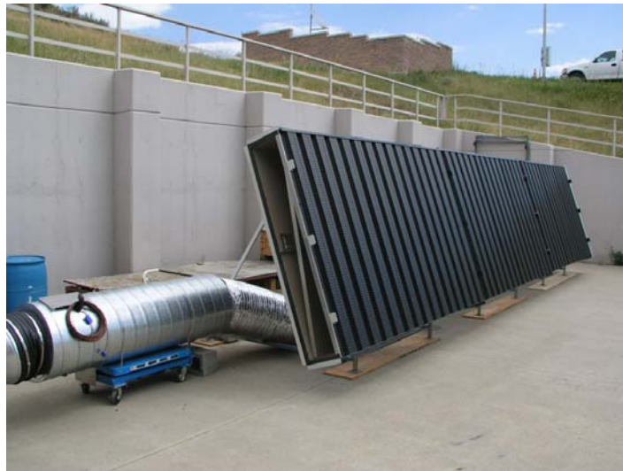
Figure 3 A prototype modular transpired solar collector under test
