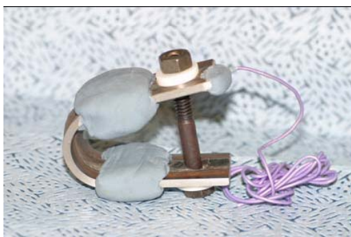
Figure 2. Prepared Polarized U-Bend Specimen, Before Bolt Tightened
