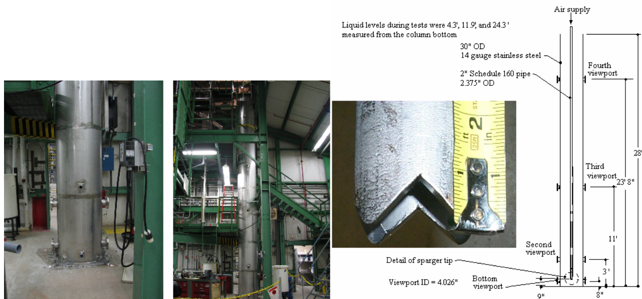
Figure 3: Bubble Column Design and Installation 1
