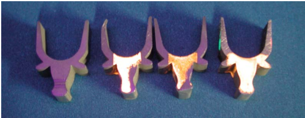
Figure 2. Armatures. Upper photo made in room light. Bottom photo made with ultraviolet illumination to produce fluorescence from the three right hand projectiles.
