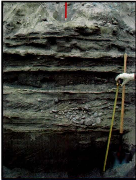
Figure 5.1. Exposed trench face showing layered heterogeneity in Hanford's 200 East Area (Ward et al., 2004)
