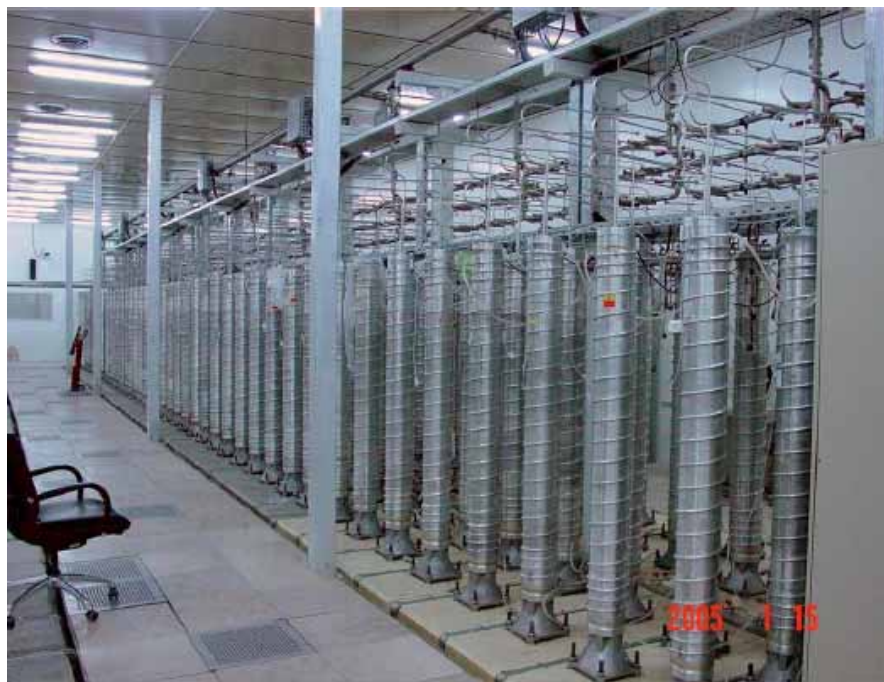
Fig. 33. 164-centrifuge cascade at the Natanz PFEP, Iran.
