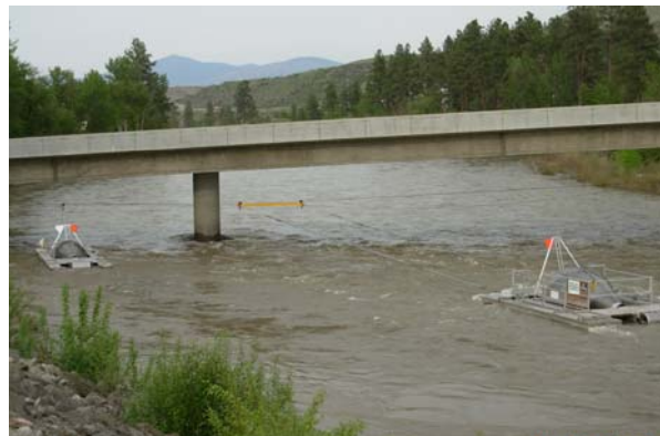
Figure 3 Photograph taken from downstream showing the 8-ft rotary screw trap in Position 1 (right) and the 5-ft rotary screw trap in Position 2 (left) at 9,500 cfs.
