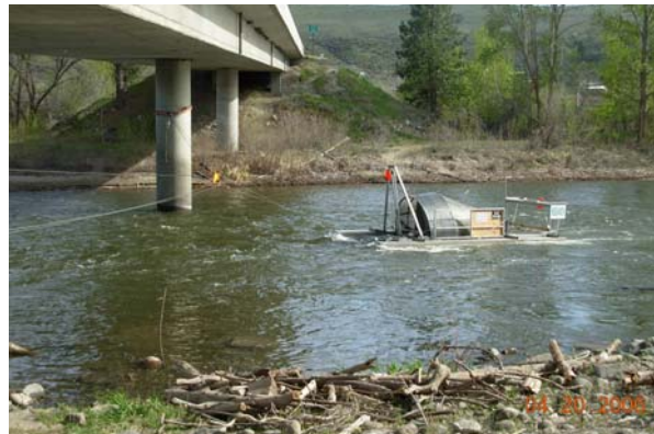
Figure 2. Photograph taken from the west bank showing the 8-ft rotary screw trap deployed in Position 1 at 2,050 cfs.
