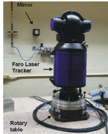
Fig 8: Faro laser tracker test setup
