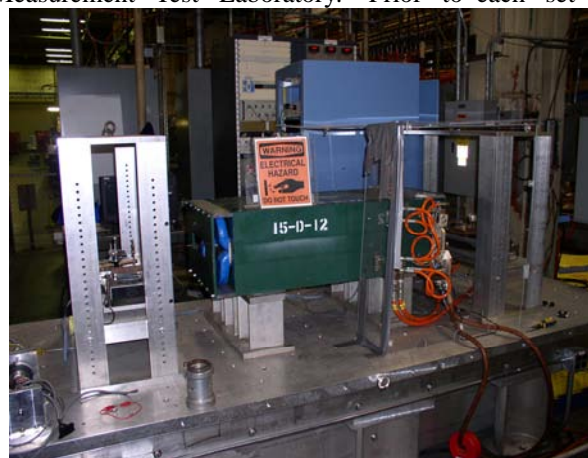
Figure 2: 10D37 dipole magnet on the test bench.
