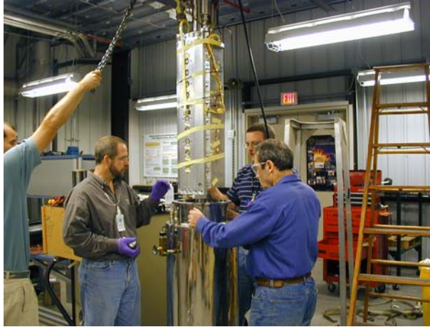
Figure 8-6: 1000 hp HTS field coil being lowered into test fixture at ORNL.
