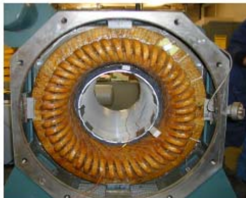
Figure 3: Photo showing the aluminum cylindrical shell in the 1000-hp stator.
