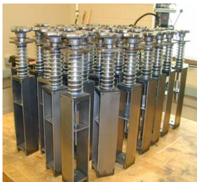
Figure 9-2: Creep test fixtures.
