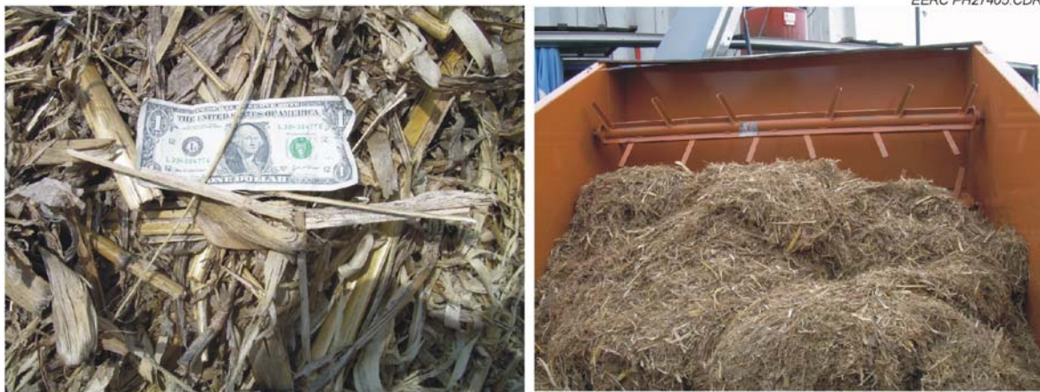
Figure 18. Corn stover before reduction in size (left) and after size reduction (right).
