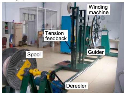
Fig. 4. The layout of solenoid magnet winding machine
