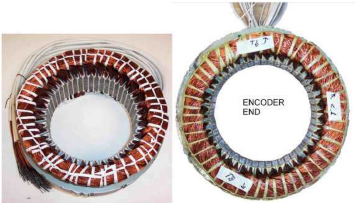
Fig. 43. Stator before (left) and after (right) rewinding.
