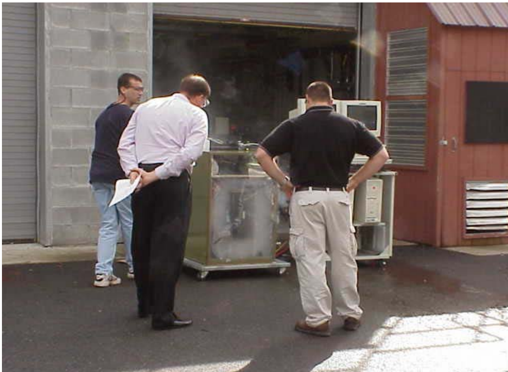
Figure 14: Successful Pass of UL Smoke Testing Demonstrating Ventilation and Air Changes
