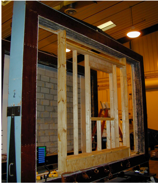
Figure 3. Wall framed to accept window, mounted in RGHB test frame
