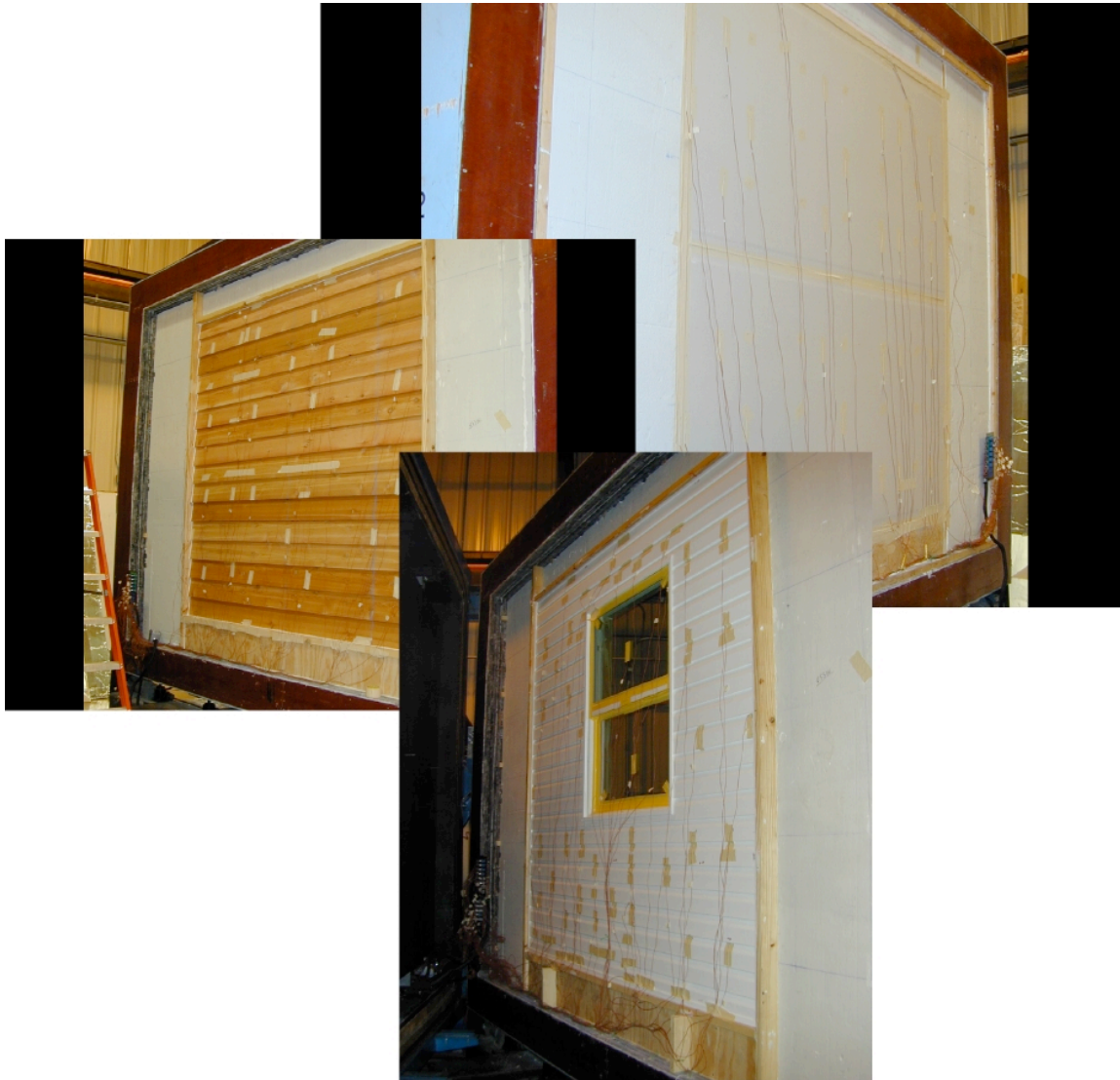
Figure 6. Photographs showing thermocouple placement on clear wall front and back and on interior wall with a window.
