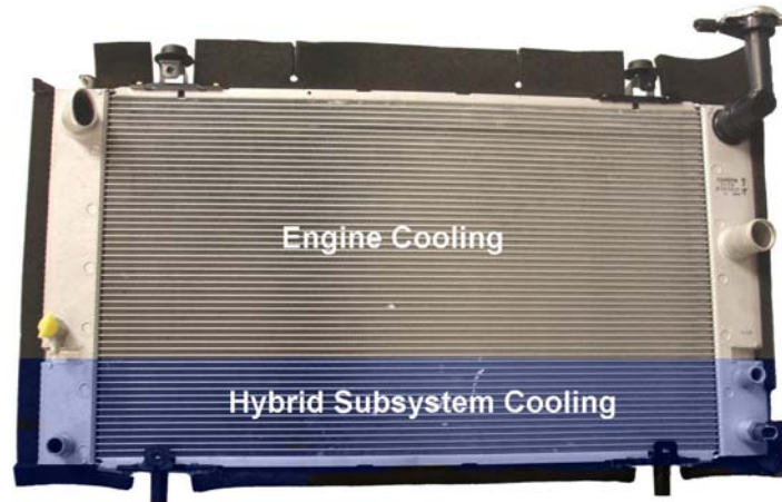
Fig. 5.10. Radiator for Prius engine (upper) and hybrid subsystems (lower).
