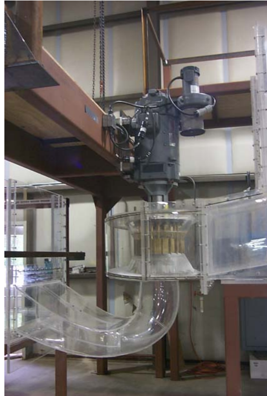
Figure 2- 3. Observational 1:25-scale physical model of the Ice Harbor turbine at the U.S. Army Engineering Research
