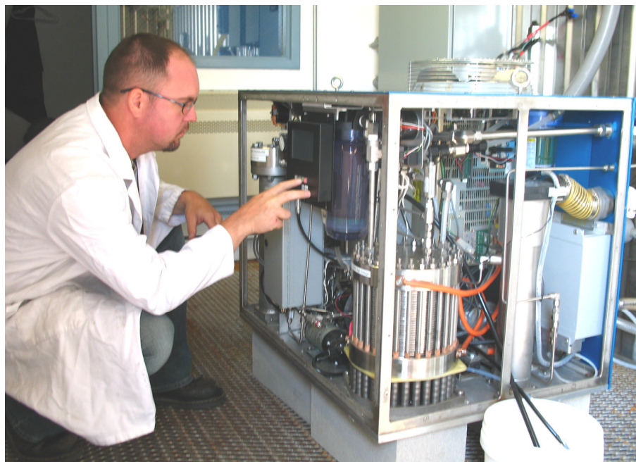
Figure 11. GES EP-1 Electrolyzer Installed at NREL Test Facility (Photo courtesy of Kevin Harrison, NREL)
