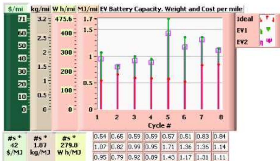
Fig. 23. Average EV battery energy demand, weight, and cost per mile with ideal base 9-turn motor and 9-18 turn-switching motor prime-movers.
