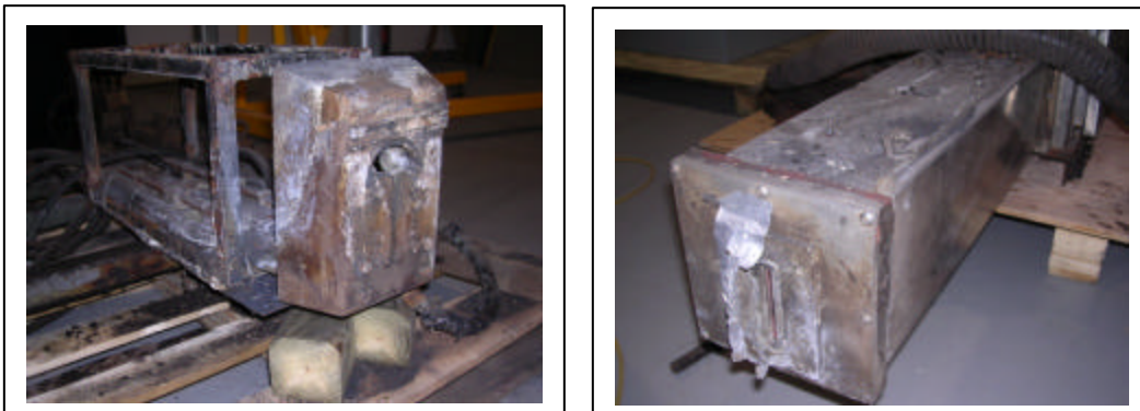
Condition after Tests, external (left) and internal (right). Components, particularly the exterior, showing effects of harsh environment.
