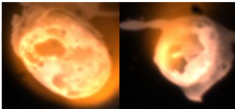
Figure 36: Large Voids during Char Burning, Very Large Droplet of Black Liquor A, 95% Solids, in 800 °C Air
