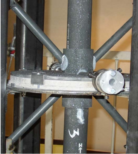
Figure 97 Window section with optical accesses in three orthogonal directions
