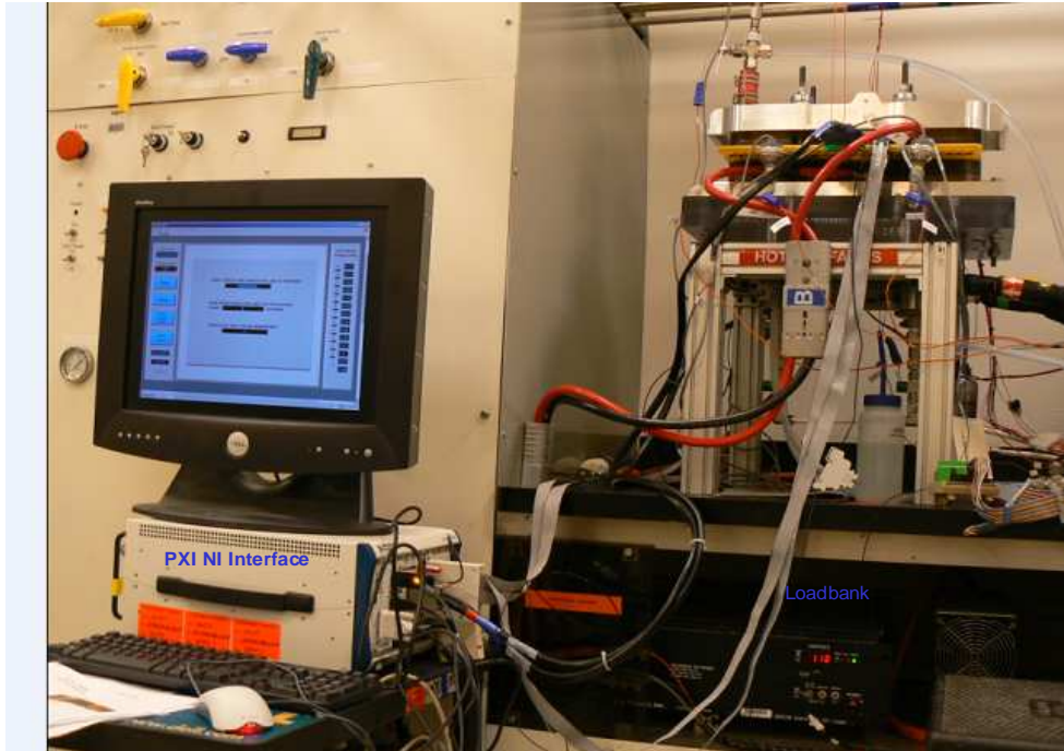
Figure 350. Fuel Cell Module Interface with PXI NI Interface
