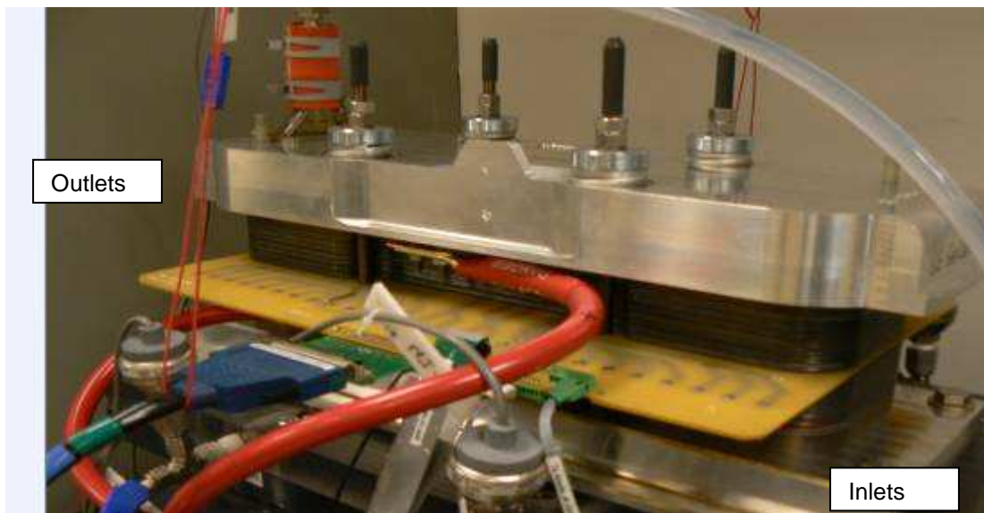
Figure 349. Fuel Cell Module showing segmented approach at cell 7/8 interface.
