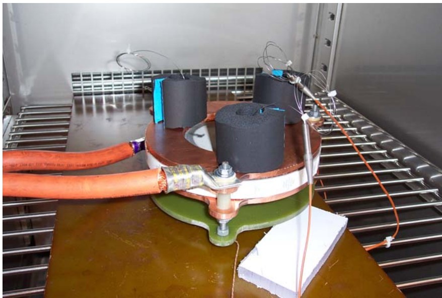
Fig. 2.21. SBE 580 \mu\text{F} film capacitor test fixture inside environmental chamber.
