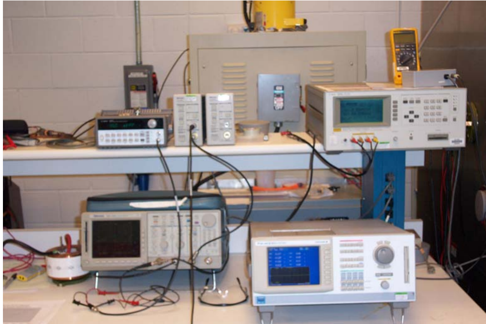
Fig. 2.3. Instrumentation for the capacitor tests.
