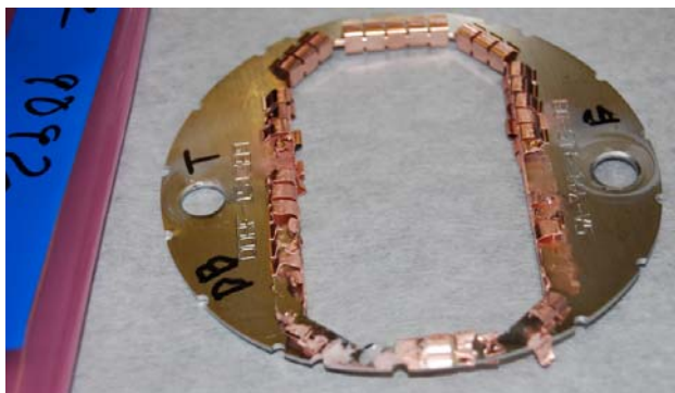
Figure 8: Melted omega seal of the 9092-flange.
