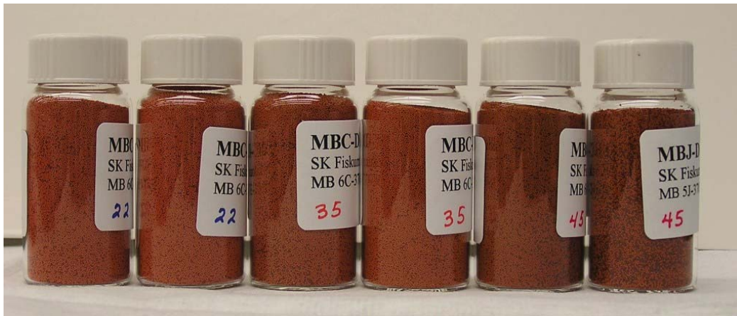
Figure C.2. Microbeads 6C-370/745 Resins Stored Dry at Ambient Temperature, 35°C and 45°C, from left to right: MBC-DL-1, MBC-DL-2, MBC-DM-1, MBC-DM-2, and MBC-DH-1, MBC-DH-2
