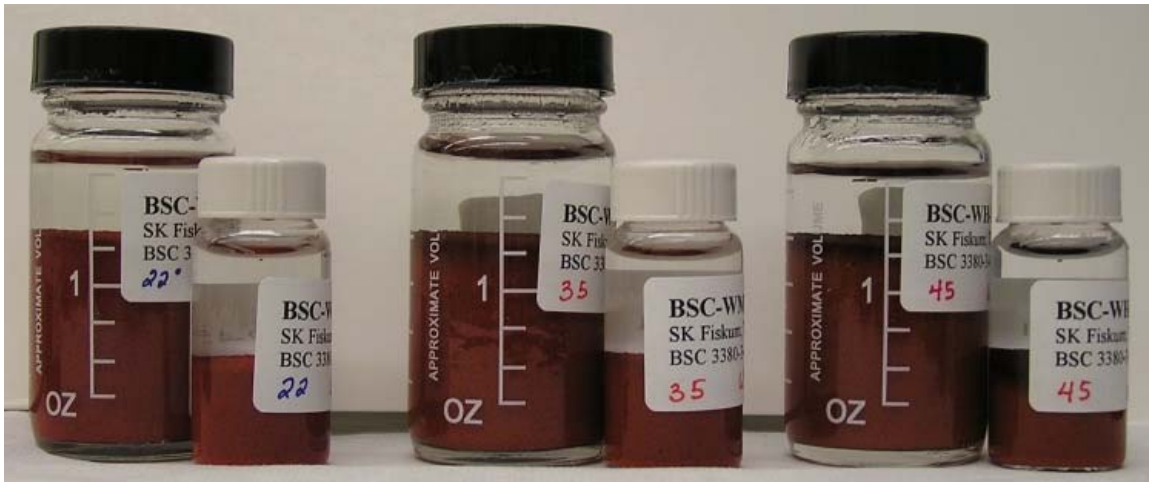
Figure C.3. Boulder Scientific Corporation 3380-3-0200 Resins Stored Wet at Ambient Temperature, 35°C and 45°C, from left to right: BSC-WL-1, BSC-WL-2, BSC-WM-1, BSC-WM-2, and BSC-WH-1, BSC-WH-2
