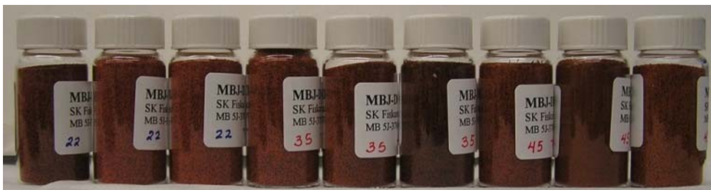
Figure C.6. Microbeads 5J-370/686 Resins Stored Dry at Ambient Temperature, 35°C and 45°C, from left to right: MBJ-DL-1, MBJ-DL-2, MBJ-DL-3, MBJ-DM-1, MBJ-DM-2, MBJ-DM-3, MBJ-DH-1, MBJ-DH-2, and MBJ-DH-3
