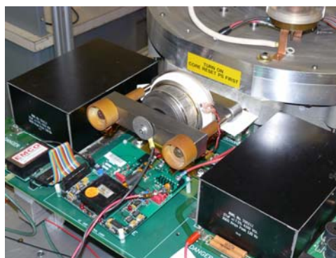
Figure 8: Photograph of the single device test stand with a press-pack IGBT.
