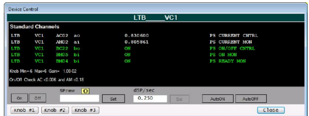
Fig.5. MPS Control Panel
