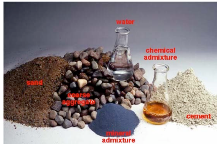
Figure 3.1 Basic concrete constituent materials
