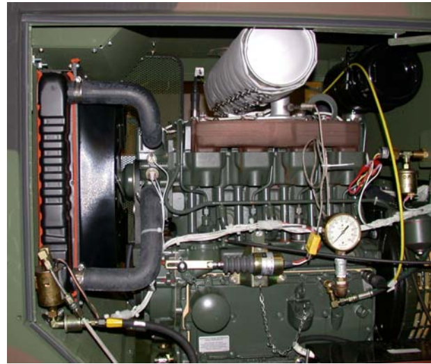
Figure 1: Pictures of the U.S. Army's Tactical Quiet Generator (TQG), showing an external view (top left); an interior view (top right); another interior view (bottom right), including a portion of the generator enclosure in the lower right corner of the picture; and the accelerometer location on the generator enclosure (bottom left) with the yellow arrow pointing to the accelerometer. Pictures are courtesy of the U.S. Army Research Laboratory.
