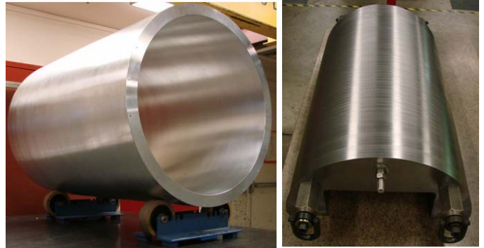
Fig. 6. Aluminum shell and iron yoke laminations.
