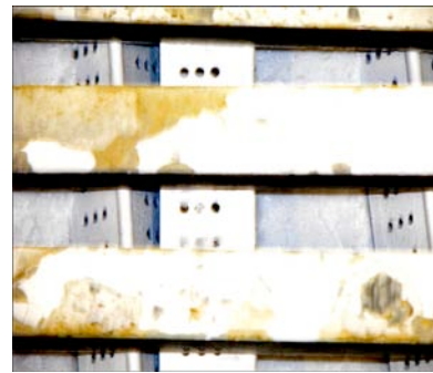
Figure 5.39 Closeup of specimens after 18-month exposure in solution of \text{Ca}(\text{OH})_2 .
