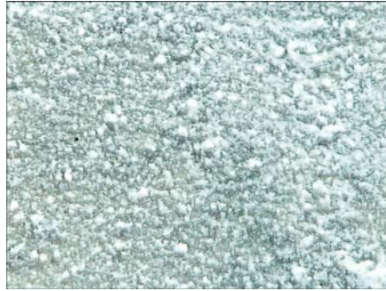
Figure 5.46 Carbonate crystal deposits on surface of specimen cured in \text{MgHPO}_4 .
