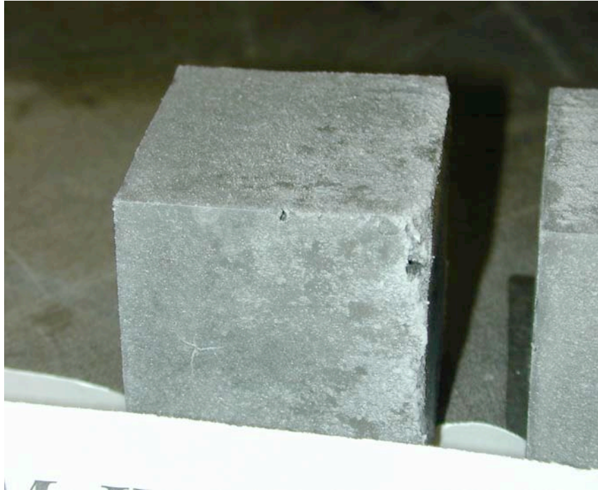
Figure 5.7 Cube specimen after 1 month in \text{MgHPO}_4 .
