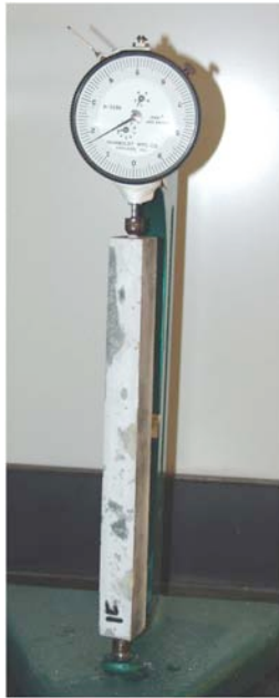
Figure 5.2 Length change test setup.
