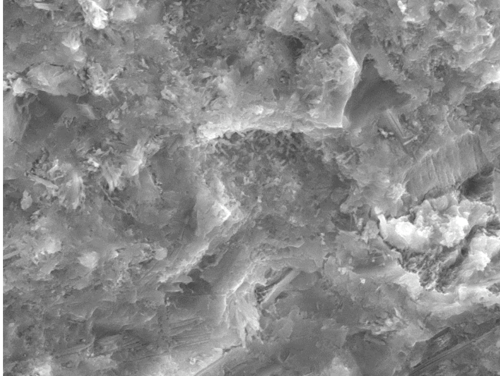
Figure 5.18 SEM of sample cured in \text{MgHPO}_4 solution for three months. The paste contains C-S-H, \text{Ca}(\text{OH})_2 and ettringite crystals (X 4000).
