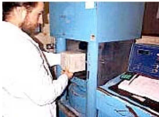
Figure 5.4 Representation of compressive strength test of cube test specimen.
