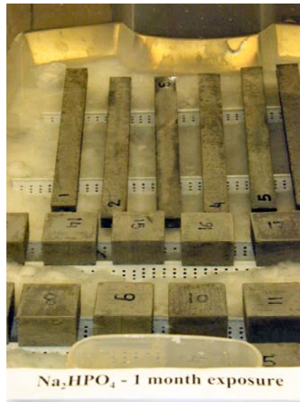
Figure 5.5 Exposure testing in saturated brines in which PVC corner braces are used to suspend cubes and prisms above the excess solids (visible).
