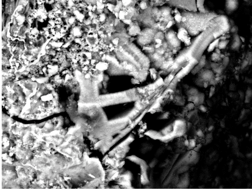
Figure 5.22 Same area (as in Fig. 5.21) in backscattered electrons. The whiter zones are rich in phosphorous (X 2000).
