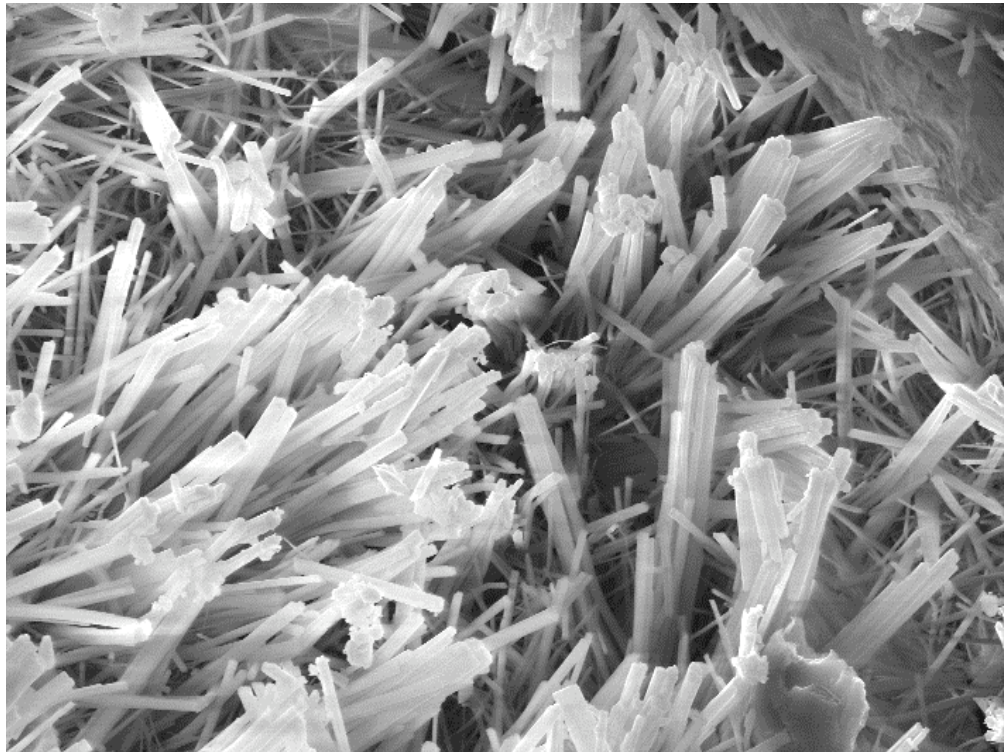
Figure 5.19 Locally, some pores are filled with well developed needles of ettringite (X 2000).
