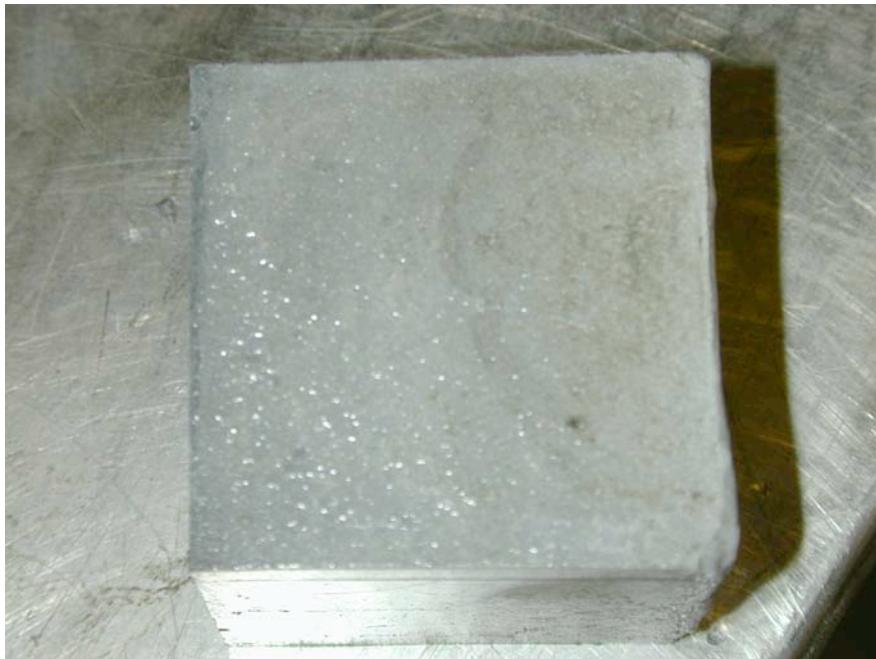
Figure 5.8 Cube specimen after 1 month in \text{Na}_2\text{HPO}_4 .
