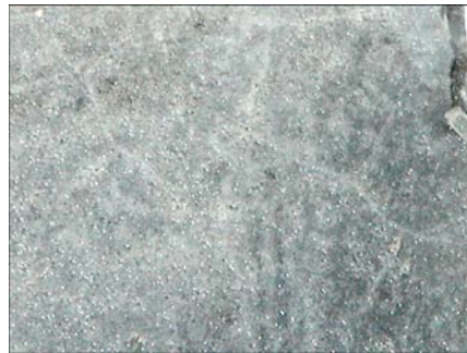
Figure 5.43 Carbonate crystal deposits on surface of specimen cured in \text{Na}_2\text{HPO}_4 .
