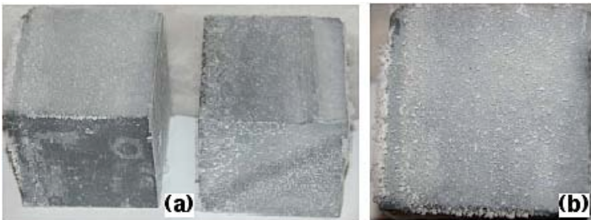
Figure 5.25 Crystals of \text{Ca}(\text{CO})_3 present on cube specimens stored in \text{Ca}(\text{OH})_2 solution 12 months.
