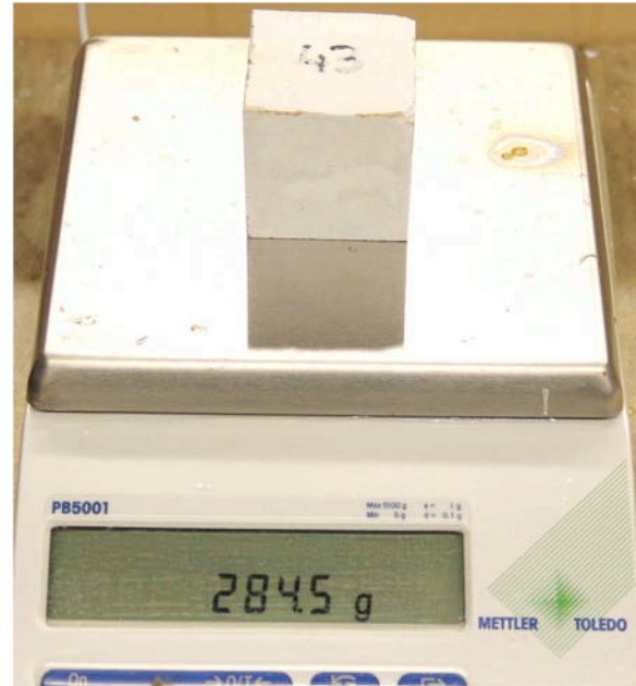
Figure 5.3 Specimen weight determination.
