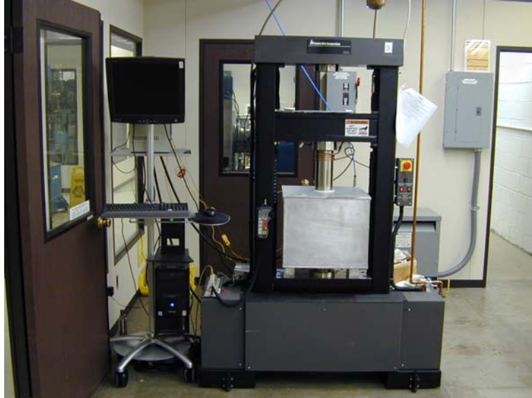
Figure 11. Picture of Modified Gradient Stress Relaxation Test Frame
