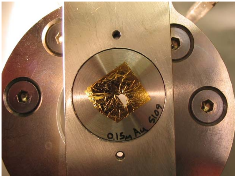
Figure 21. Picture of the gold target foil after interaction with the NDCX beam. The outer diameter of the foil holder ring is 17 mm and the inner diameter is 5 mm. The hole is approximately 2.3 by 1.1 mm.
