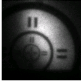
Figure 19. Profile of the beam on a scintillator placed at the target location. The distance between the two marks outside the innermost circle is 1 mm.
