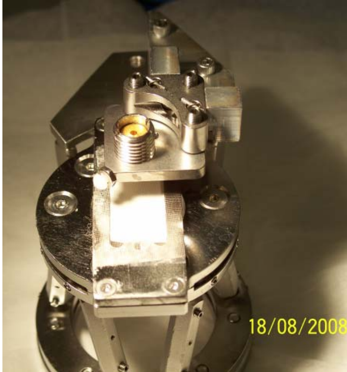
Figure 26. Gold cone with alignment fixture for test of concentration effect of cone using scintillator.
