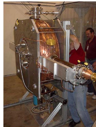
Figure 16: 201-MHz MICE prototype cavity installed in the MuCool Test Area at Fermilab.
