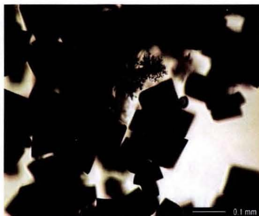
Fig. 3. Micrograph of a melter-bottom sludge (spinel and silver) [10].
