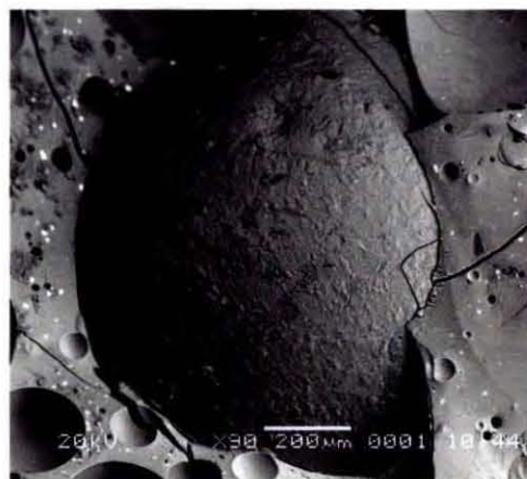
Fig. 4. Scanning electron Microscopy (SEM) image of sulfate bubble in an LAW glass [8].
