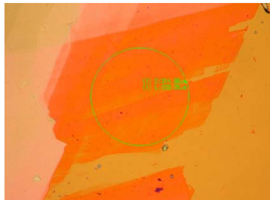
Fig. 1 Large (~200X150μm) flake of four and five-layer graphene on 400 nm thick SiO 2 . Circle ( \phi=100\mu\text{m} ) represents a typical spot size of the photon beam in an ARPES experiment.
