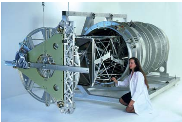
Figure 1.6. ATK's FAST Mast enables rapid deployment of the RF transmission tower [21].
