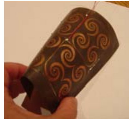
Figure 2.1. (a) Measured rectified DC power as a function of the DC load for different incident power levels. A photograph of dual-polarized 2.4-GHz patch rectenna is shown in the inset. (b) A broadband rectenna array on a flexible substrate (no ground plane, bidirectional).
