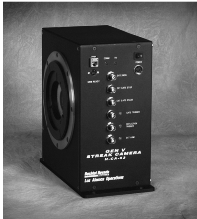
Figure 2. The Generation V Camera. The camera has few hardware controls or indicators and requires an Ethernet communication link and a wall-mounted power supply.
