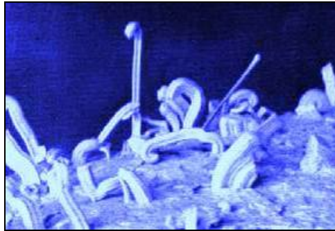
Figure 19. Close-up of tin whiskers
