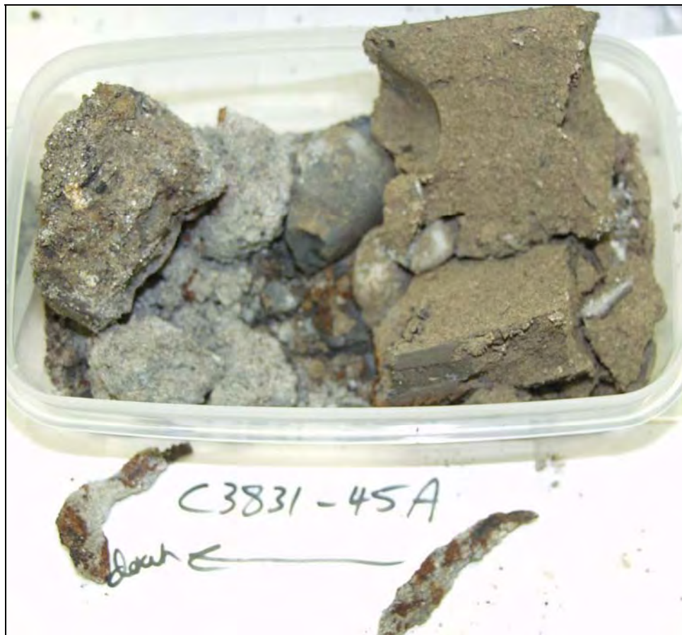
Figure 2.20. Rusted Metal Fragments from Backfill Material in C3831. Metal fragments came from 46 ft depth. The top of the 0.5-ft core is to the right.
