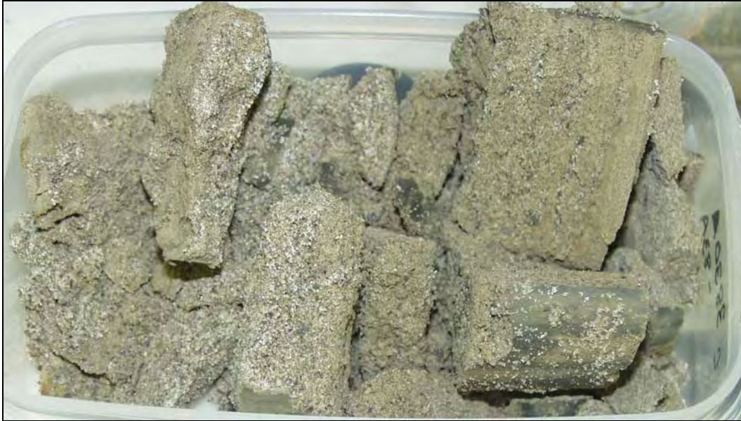
Figure 2.29. Hanford Formation H2 Unit in C3832 - Core C3832-83A. Alternating layers of slightly moist, well laminated, moderately to well-sorted, loose, grayish-brown, medium sand (S), and moist, compact, strongly calcareous, light olive-brown, silty fine sand (mS). The top of the 0.5-ft-long core is to the right.
