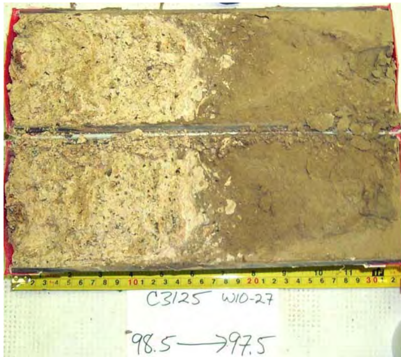
Figure 2.7. Sharp Contact Between the Upper and Lower Cold Creek Subunits in Borehole 299-W10-27. The upper unit consists of unconsolidated, yellowish-brown, silt and fine sand (mS), in sharp contrast to the white, CaCO 3 -cemented lower unit. The top of this 1-foot core is to the right.
