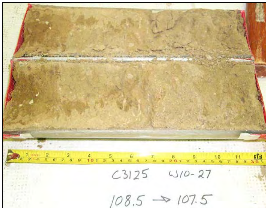
Figure 2.11. Lower Cold Creek Subunit (CCU l ) in 299-W10-27. Massive to mottled, poorly sorted, sand and silt [(g)mS] with white stringers and nodules of secondary, pedogenic, calcium carbonate. The top of the core is to the right.
