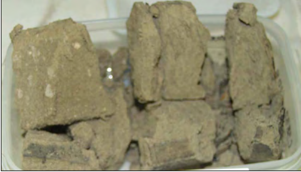
Figure 2.30. Upper Cold Creek Unit in C3832 - Core 3832-110B. Described as slightly moist, laminated, well-sorted, strongly calcareous, olive-brown, silty fine sand (mS). Whitish \text{CaCO}_3 -cemented nodules to the left are associated with the underlying caliche of the lower CCU. The top of the 0.5-ft core is to the right.
