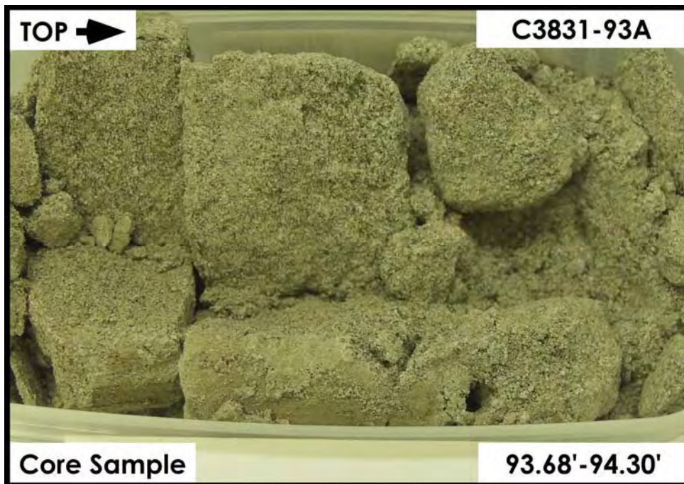
Figure A-3.32. Hanford Formation (H2 unit) 93.68 ft – 94.30 ft
