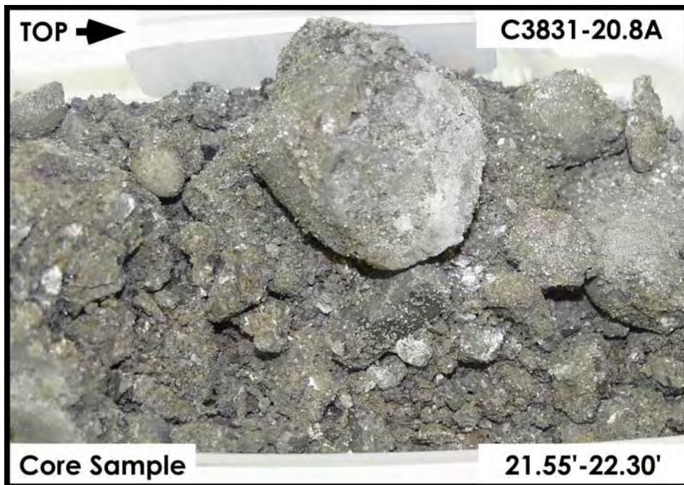
Figure A-3.4. Backfill 21.55 ft – 22.30 ft
