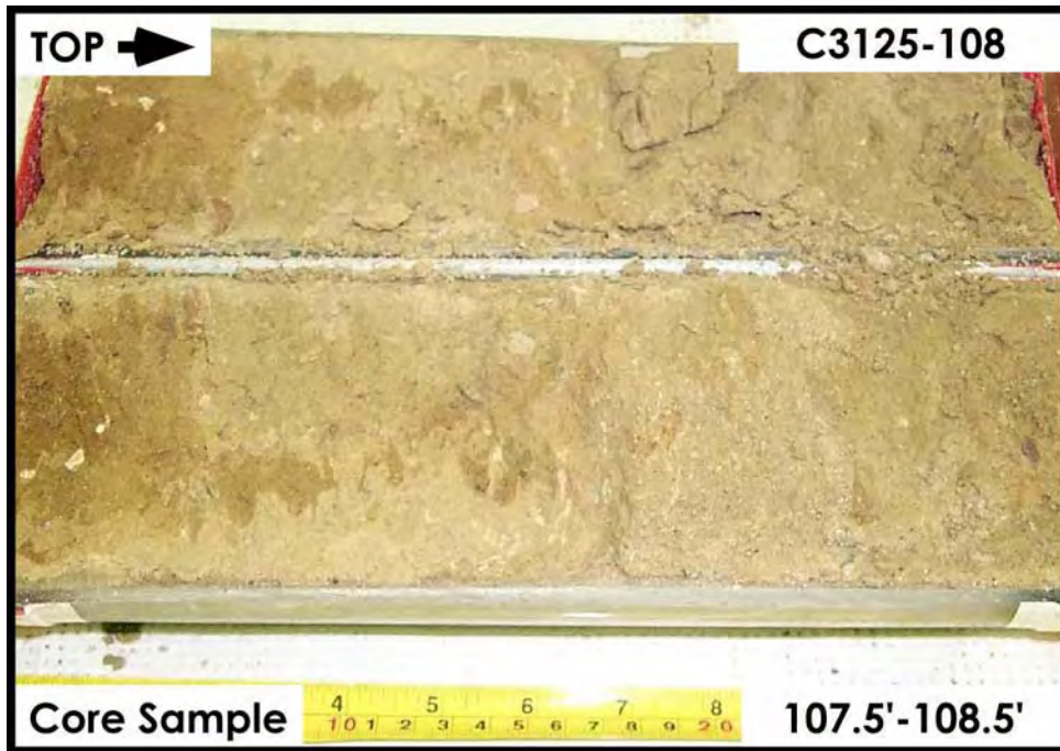
Figure A-1.39. Cold Creek Unit – Lower (CCU l ) 107.5 ft – 108.5 ft
