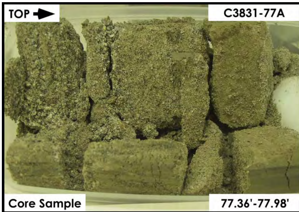
Figure A-3.24. Hanford Formation (H2 unit) 77.36 ft – 77.98 ft
