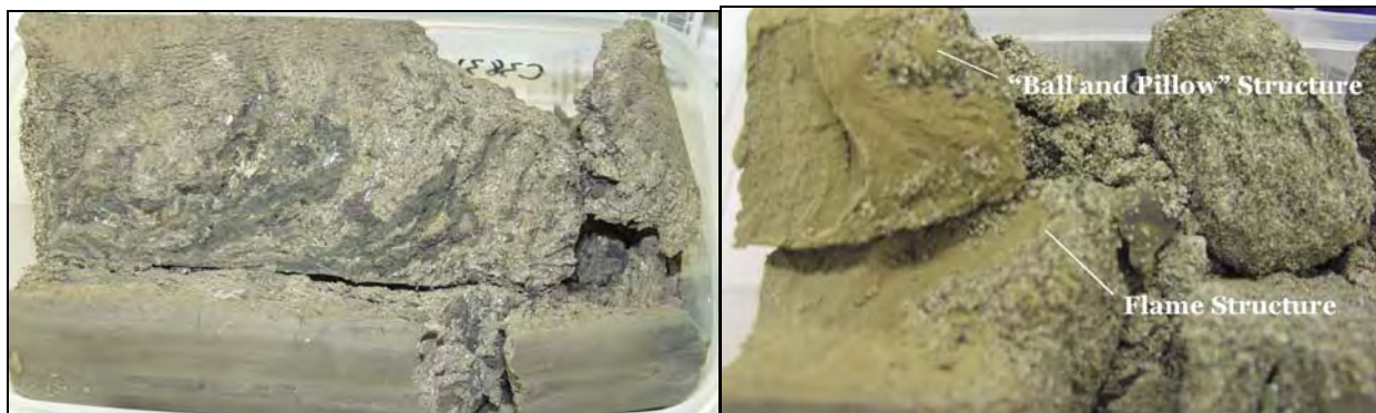
Figure 2.23. Soft-Sediment Deformation Within the Hanford Formation H2 Unit. Left Photo: Core C3831-60B, 0.5-ft long. Moist clastic dike, with alternating sub-vertical layers of sand, silt, and clay. Right Photo: C3831-85B, 0.3-ft long. Syndepositional loading and deformation occurred along the contact between slightly moist, fine to medium sand (above) and moist silt (below). The tops of the cores are to the right.
