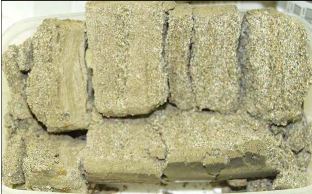
Figure 2.22. Interbedded, Laminated Sand and Silt Near Base of the Hanford Formation H2 Unit - Core 3831-97A. Slightly moist, loose, fine to medium sand (S) is interbedded with more cohesive silty fine sand (mS) to silt (M) layers.
