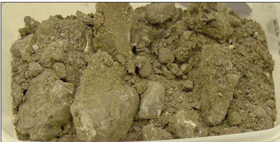
Figure 2.13. Typical Backfill from Borehole C3830. Core sample C3830-27.91A, described as a slightly moist, dark grayish brown, poorly sorted, pebbly, fine to coarse sand (gS), weakly to moderately calcareous. The top of the 0.5-ft core is to the right. Considerable pulverization of the sample occurred during drilling, as indicated by the abundance of angular gravel clasts.
