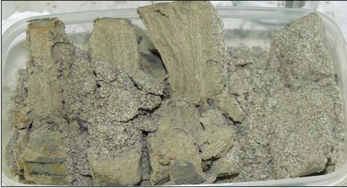
Figure 2.15. Interbedded Sand and Silty Sand Within the Hanford Formation H2 Unit. Core C3830-58.29A, described as two lenses of slightly moist, cohesive, brown, well-sorted and laminated silty fine sand (mS), interbedded with loose, grayish-brown, medium-grained sand (S). The top of the 0.5-ft core is to the right.
