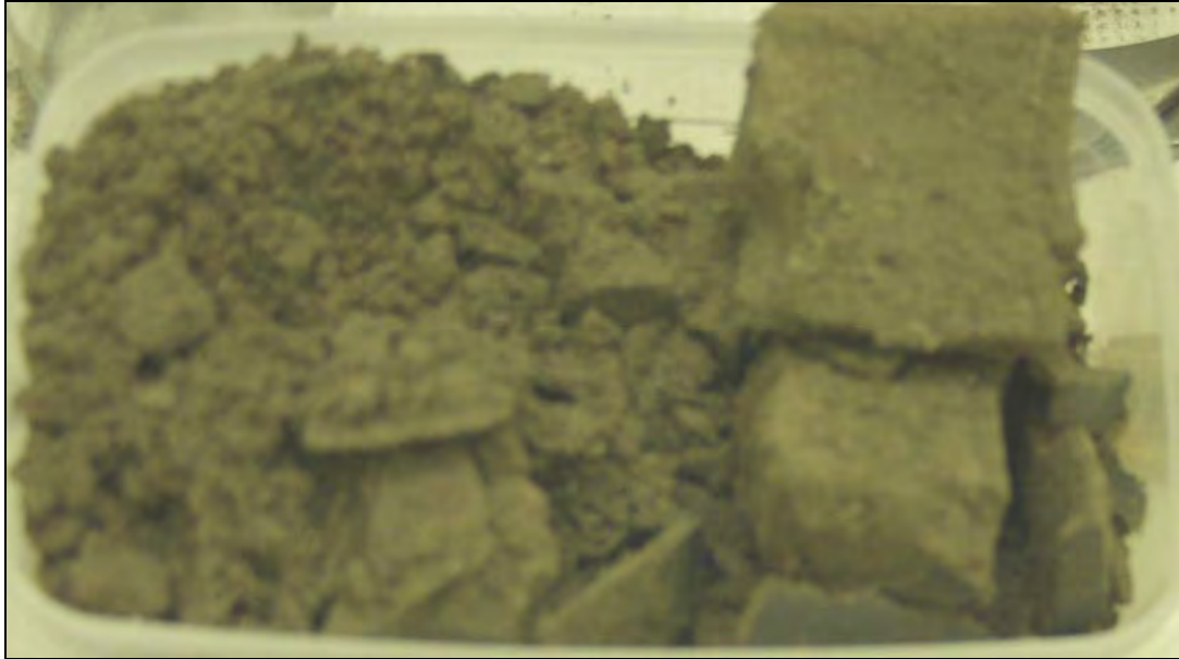
Figure 2.28. Fine-Grained Sediments at Base of Backfill Sequence - Core C3832-44A. Described as a moist, consolidated, well-sorted, strongly calcareous, dark grayish-brown, felsic, silty fine to very fine sand (mS). The top of the 0.5-ft core is to the right.
