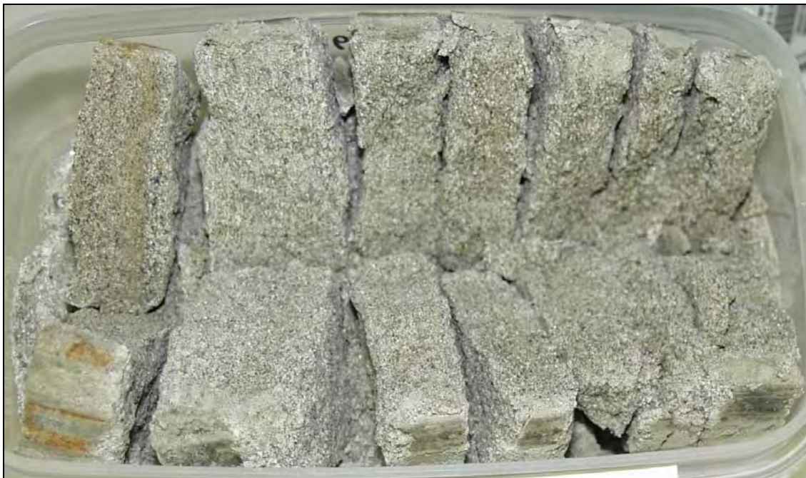
Figure 2.14. Fine to Medium Sand Recovered from the Hanford Formation H2 Unit in Borehole C3830. Core C3830-76.98A, described as slightly moist, light gray, well-sorted, fine to medium sand (S), moderately calcareous. The core separated along natural, well-developed laminations. The top of the 0.5-ft core is to the right.
