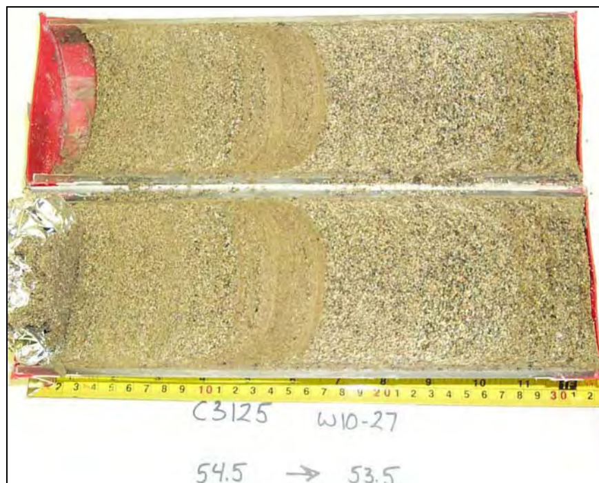
Figure 2.10. Hanford Formation H2 Unit in Borehole 299-W10-27. A thin (0.2 ft) layer of well-laminated silty very fine sand (mS) lies between beds of medium- to coarse-grained “salt and pepper” sand (S). One of the nine characterization samples from this borehole was collected from the silty sand layer at 54.2 ft. The top of the core is to the right. Notice the drilling-induced drag folding along the sides of the core.
