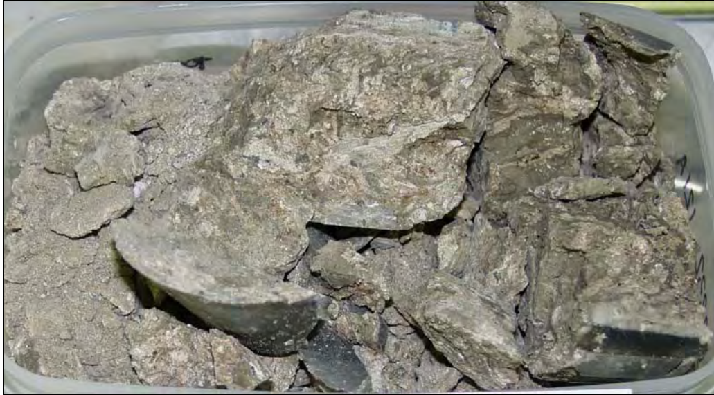
Figure 2.31. Lower Cold Creek Unit Within C3832 - Core C3832-121A. Described as slightly moist, very poorly sorted, mottled to massive, strongly to very strongly calcareous, strongly consolidated, olive, pebbly sandy mud (gsM), mottled with gray to brownish-gray, pedogenic, calcium-carbonate-cemented caliche nodules and stringers. Includes about 10% small pebbles. The sample in the tray was broken apart during removal from the core liner. The top of the 0.5-ft core is to the right.
