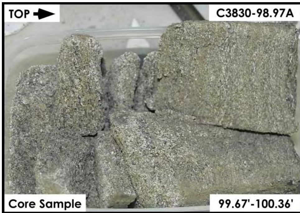
Figure A-2.28. Hanford Formation (H2 unit) 99.67 ft – 100.36 ft
