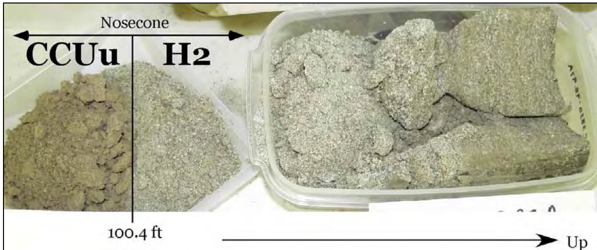
Figure 2.16. Contact Between Hanford Formation H2 and Cold Creek Units. Contact was encountered in the nose cone of the splitspoon sampler in core #3830-98.7. The contact is well-defined based on the sudden textural, color, and moisture change at 100.4 ft bgs. The Hanford formation H2 unit is described as slightly moist, laminated, moderately sorted, light brownish-gray, fine to coarse sand (S). The underlying CCU u unit is described as moist, well-sorted, yellowish-brown, silty fine sand (mS). The top of the core is to the right.
