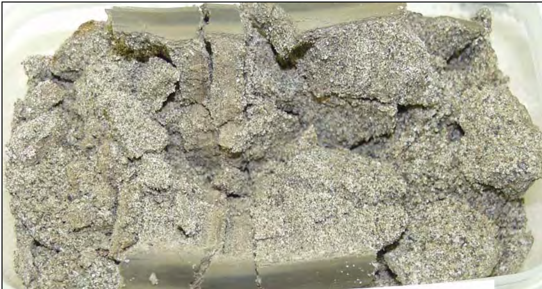
Figure 2.21. Hanford Formation H2 Unit in C3831 - Core C3831-69A. Mostly a slightly moist, loose, well-sorted, laminated, moderately calcareous, medium to coarse, “salt and pepper”-like, grayish-brown sand (S). A few thin lenses of brownish, silty fine sand (mS) are interspersed. The top of the 0.5-ft-long core is to the right.
