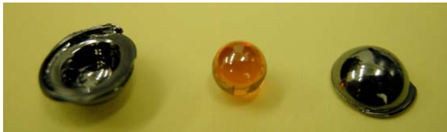
Figure 13. IG3 Hemispherical Shells Shown Flanking a GLS 5-mm Spherical Core
