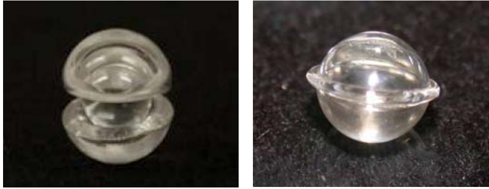
Figure 12. Picture Sequence Showing the Assembly of the Clad Ball. The hemispherical shells are arranged around the core (left) and pressed to yield the final assembly (right).
