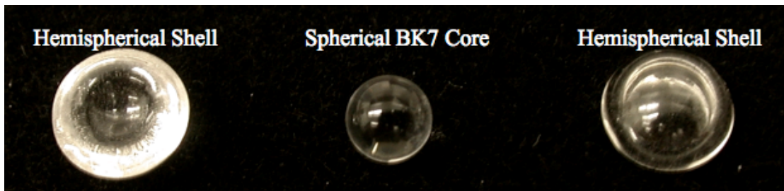
Figure 11. Images Showing the Sequential Steps Required to Produce a Clad Ball by Using Super Vidron for the Shell and BK7 Glass for the Core. The hemispherical shell at the left is oriented to be concave while the hemispherical shell at the right is oriented such that its convex surface faces the camera.
